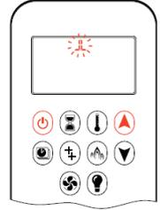
**NB!** Once the pilot flame is confirmed, the motor will automatically go to maximum flame height.
