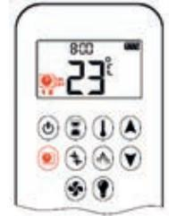
**NB!** The set temperature for Thermostat mode is the temperature for the operating time in Program mode. If the set temperature for Thermostat mode is changed, the temperature for the operating time in Program mode is also changed.
